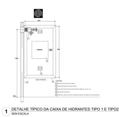
1 DETALHE TÍPICO DA CAIXA DE HIDRANTES TIPO 1 E TIPO 2 SEM ESCALA
